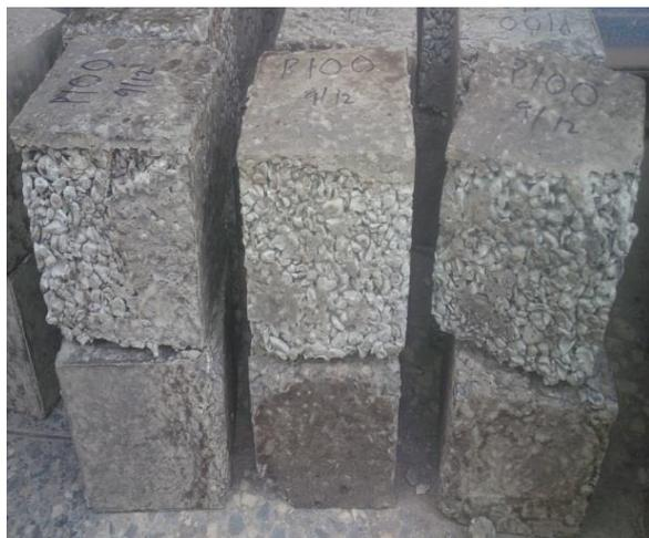
Figure 8d. Normal concrete (lower row) and 10% PKS (upper row) at 400°C
