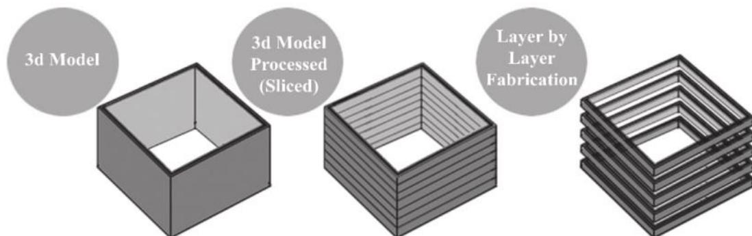
Figure 3. Additive manufacturing (AM) process [18]
