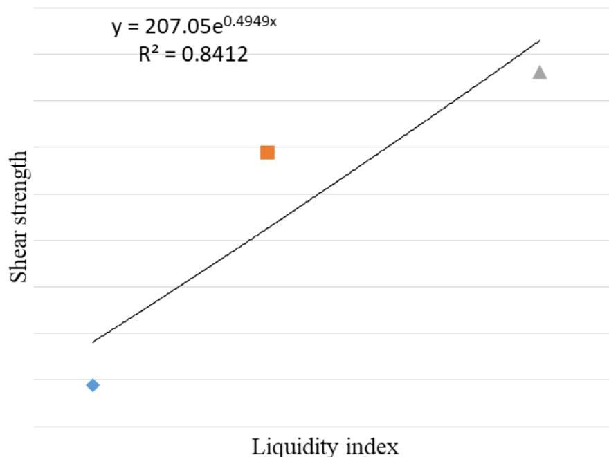
Figure 4.3. Exponential regression graph for shear strength and liquidity index
