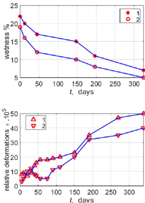
Figure 2. Dependence of deformations on moisture changes – 1 – block, 2 - panel
