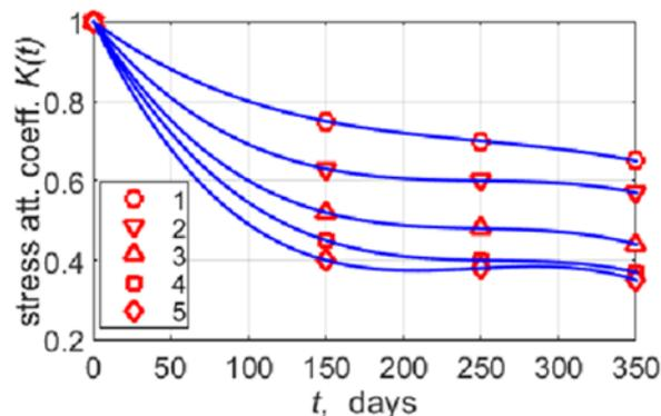
Figure 1. Dependence of stress attenuation coefficient on the creep characteristics of concrete and the duration of development of non-stationary forced deformation
