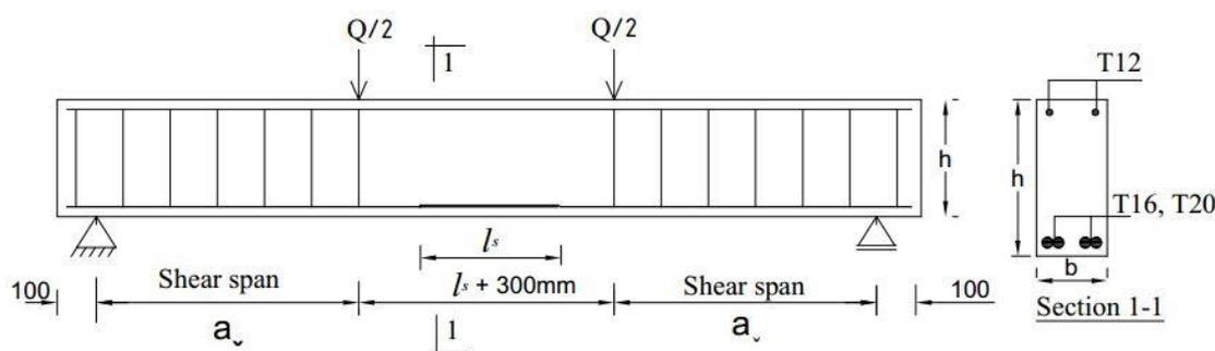
Figure 1. Typical beam without stirrup over lap.
