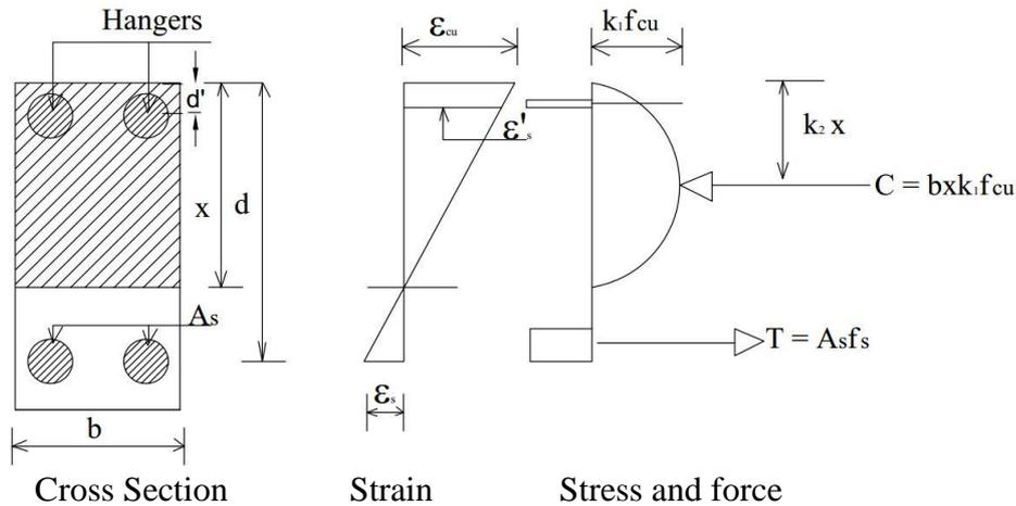
Figure 2. Strain and stress distribution at failure.
