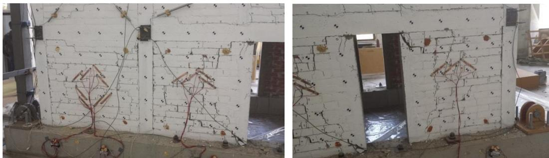
Figure 8. Damage to the infill of MODEL 2
