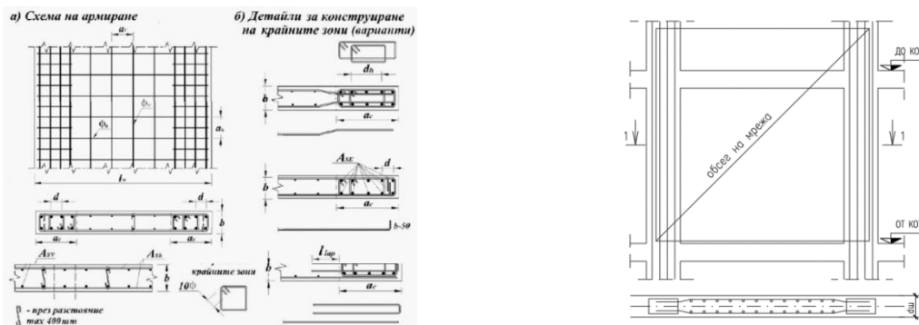
Figure 12. Shear wall detailing from ПД-02 (left image) (a) [8] detailing given by E. Boychev (right image) (b) [2]
